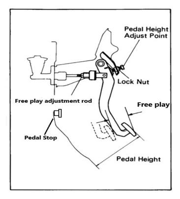
It is imperative for the performance and life of your clutch, that the clutch pedal is adjusted once a new clutch is fitted <u>and</u> regularly checked and re-adjusted!
