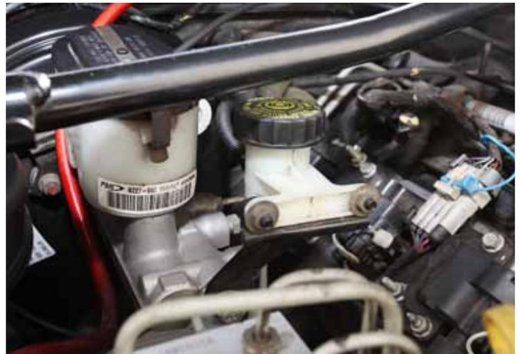
**STEP 14** The hydraulic clutch needs to be bled of air bubbles, just like a brake system. This is a messy job on the Holden T56, as the bleed nipple is located inside the bellhousing (see bleed nipple, Step 5), making it difficult not to get fluid everywhere. Due to the tiny size of the reservoir it will need topping up several times, so watch it like a hawk during bleeding. If it runs dry, air will re-enter the system and you'll have to start over.
