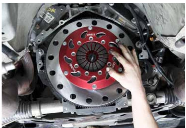
**STEP 09** Machined components often have a very light anti-corrosion film to keep their surfaces pristine until installation. Clean off this film and any fingerprints with a quick squirt of brake or carby cleaner, as either can lead to clutch slippage or uneven and premature wear. It's imperative that the clutch plates are installed in their correct orientation (they're clearly marked) otherwise they will foul the floater and apply plates.
