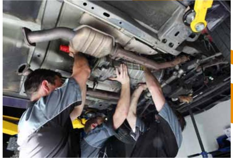
**STEP 12** Line up the dowels, tweak the position gently and the 'box should slot straight into place. If it hangs up, don't let the weight of the 'box sit on the clutch plate as it will shift it out of alignment or, worse still, bend the clutch plate. Never force it; the 'box should seat by hand. Once in, it's fine to use a couple of bolts to hold it in place but never use the bolts to pull it into position, as this can break the bellhousing or damage the new clutch.
