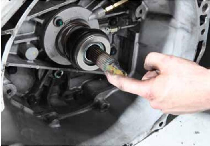
**STEP 11** Put a smear of high-temperature grease on the snout of the input shaft and a small amount on the front edge of the input spline — the clutch plate will push it down the spline when the 'box is slipped into place. Don't apply too much or it could fly out and you'll risk contaminating the friction surfaces, which is bad. Before refitting the 'box, check the block face and the bellhousing for any crud that could cause a misalignment.
